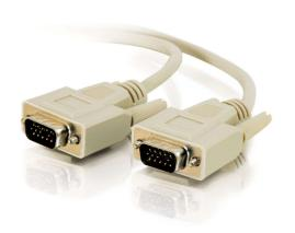
This cable is constructed from 28 AWG wire, and is foil shielded to protect short cable runs from EMI/RFI interference. The fully molded connectors have easy-to-use extra long thumbscrews for a fast connection. Use this cable for video presentations, classroom environments or just for organizing a work area for maximum comfort and efficiency.
