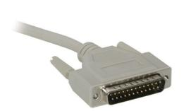
Easily extend your cable at a lower cost than buying a new cable. All 25 lines are wired straight through pin-to-pin for ease of compatibility. Each cable is foil shielded for EMI/RFI protection, and is available fully molded with thumbscrew connectors for a fast, easy connection every time.
