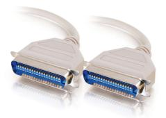
Gain flexibility and efficiency by positioning your printer in the best location (up to 50 feet away) by using our superior quality, Centronics-style cable. This male/male will connect a Centronics switch box to the parallel printer. Each cable is fully molded and foil shielded to block EMI/RFI interference caused by a noisy office environment.
