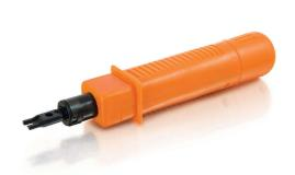
This impact punchdown tool has an impact mechanism inside divided from the turnable body. It also has a rugged frame with a storage compartment in the tool's body for storing one blade. Made from hardened SNCM-21, the blade is interchangeable and reversible - very convenient. Plus, you can quickly change the blade without using a screwdriver.
