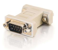
Convert a serial cable into a null modem cable with this handy adapter, a quick and easy fix for your DTE or DCE incompatibilities. Crossing the data transmission lines in straight-through serial cables, this adapter will connect two RS-232 serial ports. The adapter's molded design provides a solid connection while shielded against outside EMI/RFI interference.
