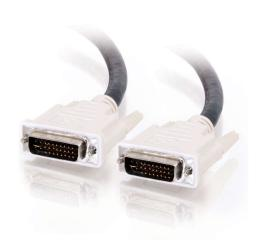
This precision-engineered cable is fully compliant with the DVI standard defined by DDWG (Digital Display Working Group). The DVI-I dual link configuration provides enough bandwidth for resolutions up to 2560 x 1600. Three analog 30 AWG coaxial lines enable high speed analog transmission.
