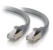
This Cat5e shielded network patch cable is an ideal solution for making a network connecting in a noisy, EMI/RFI, environment. The F/UTP shielding features an overall cable shield which provides protection from EMI/RFI noise and electromagnetic interference. This cable meets or exceeds industry standards for NEXT and return loss. The molded boot provides extra strain relief and durability. Available in a variety of colors to easily color-code your network installation.
