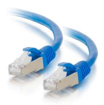
This Cat5e shielded network patch cable is an ideal solution for making a network connecting in a noisy, EMI/RFI, environment. The F/UTP shielding features an overall cable shield which provides protection from EMI/RFI noise and electromagnetic interference. This cable meets or exceeds industry standards for NEXT and return loss. The molded boot provides extra strain relief and durability. Available in a variety of colors to easily color-code your network installation.
