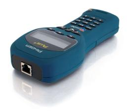
The Pinger Plus can PING using variable packet sizes and up to 99 times consecutively. In addition, PING can be performed for a single IP address, or a range of IP addresses. The Pinger Plus also identifies reversed polarity for improperly connected wire pairs, and provides a port ID feature with selectable blink rates to identify to which port on a hub or switch the wall outlet is connected.
