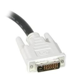
This precision-engineered cable is fully compliant with the DVI standard defined by DDWG (Digital Display Working Group). The DVI-D dual link configuration provides enough bandwidth for resolutions up to 2560x1600 pixels and allows high speed digital video transmission up to 9.9 Gbps. 28 AWG copper conductors are individually insulated in foam-polypropylene to minimize crosstalk, and ensure high speed, error-free transmission.
