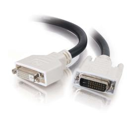
This precision-engineered cable is fully compliant with the DVI standard defined by DDWG (Digital Display Working Group). The DVI-D dual link configuration provides enough bandwidth for resolutions up to 2048 x 1536 pixels and allows high speed digital video transmission up to 9.9 Gbps. 28 AWG copper conductors are individually insulated in foam-polypropylene to minimize crosstalk, and ensure high speed, error-free transmission.
