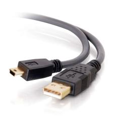
The Ultima USB cable optimizes style, quality, and value in a cable specially designed for high performance. Just plug-and-play for USB devices with the mini-b port, and this cable will deliver high speed data transfer up to 480 Mbps. Two 24 AWG and two 28 AWG heavy duty wires provide the proper current to your USB device. Dual foil and braid shielding reduces EMI/RFI interference while twisted pair construction helps reduce crosstalk thus ensuring high speed, error-free data transfer.
