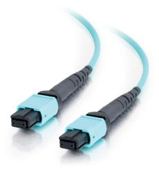
Make MTP/MPO your choice for high density fiber networks; it's specifically designed for fast ethernet, fiber channel, ATM and gigabit ethernet applications. Save time and money with MTP/MPO's increased ease of installation - simply pull one cable rather than twelve. Each MTP/MPO fiber assembly consists of twelve laser-optimized, 10G 50/125 multimode fibers under one PVC (OFNR-rated) jacket.
