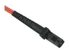
With MTRJ to SC termination, this high quality fiber optic patch cable is specifically designed for ethernet, multimedia, or communication applications. The MTRJ connector features an easy-to-use latch-type design similar to the RJ connector on a Cat5 patch cable, and is half the size of the SC connector. With its small footprint design, the MTRJ connector can increase the port density. The SC connector features a push-pull locking system.
