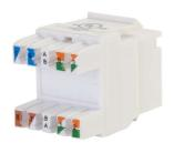
Designed for superior performance, this keystone jack is available in several colors to match housing or allow color-coded port designation in compliance with TIA-606 requirements. Includes 110-type IDC termination with strain relief caps, and comes standard with 50 µinch gold plating on the jack contacts.
