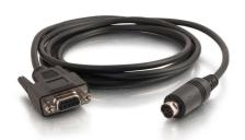
This cable is designed to provide RS-232 serial control of Mitsubishi projectors when used in conjunction with a classroom controller such as the Trulink A/V Controller (#40348). It features a standard DB9 female connector to a 8-Pin Mini-Din Male connector configured to match Mitsubishi projectors and matches the Receive (RX) and Transmitssion (TX) lines for easy installation and immediate operation.
