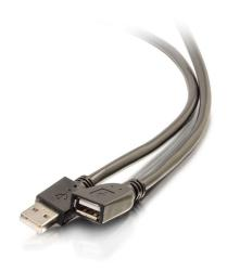
This USB Active Extension Cable is an ideal solution for USB applications which require more cable length than the 5 meter (16.5ft) length limitation of USB. This extension cable actively buffers the incoming and outgoing signals to ensure compliance with the USB 2.0 specification for electrical and timing minimums. The plenum rated jacket meets the requirements for an installation in a commercial space, and both low and high speed USB devices will function equally well with this extension.
