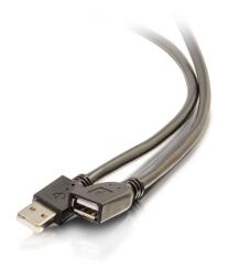
This USB Active Extension Cable is an ideal solution for USB applications which require more cable length than the 5 meter (16.5ft) length limitation of USB. This extension cable actively buffers the incoming and outgoing signals to ensure compliance with the USB 2.0 specification for electrical and timing minimums. The plenum rated jacket meets the requirements for an installation in a commercial space, and both low and high speed USB devices will function equally well with this extension.
