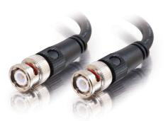
A high quality BNC cable for video applications including CCTV, broadcast, studio, boardroom presentations, home theater, etc. Manufactured from 75 0hm RG59/U dual shield coax cable (60% copper braid over foil) with a 22 AWG copper-covered steel center conductor. Finished with bright nickel-plated BNC connectors that have molded PVC strain relief to protect the cable from wear over time.
