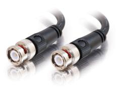
A high quality BNC cable for video applications including CCTV, broadcast, studio, boardroom presentations, home theater, etc. Manufactured from 75 0hm RG59/U dual shield coax cable (60% copper braid over foil) with a 22 AWG copper-covered steel center conductor. Finished with bright nickel-plated BNC connectors that have molded PVC strain relief to protect the cable from wear over time.
