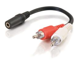
This cost-effective audio y-cable is an ideal solution for adapting your audio connections to meet your application needs. The dual conductor is shielded (26 AWG, spiral-wrapped copper shielded wire), which provides protection against EMI/RFI. The connectors are fully molded to provide excellent strain relief. Brass/nickel-plated plugs. This audio y-cable can split a signal or adapt from one connection to another.
