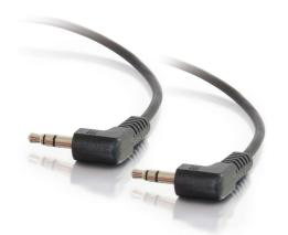
The 3.5mm right angle stereo audio cable is specifically designed for quality computer audio applications. It connects a PC sound card, MP3 player or any mini-stereo audio device with 3.5mm jacks to a multimedia speaker. This cable features two copper conductors and a drain wire. The conductors and drain wire are wrapped with a foil shield which prevents unwanted EMI/RFI interference. Fully molded nickel-plated connectors provide excellent strain relief for durable use.
