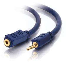
Specifically designed to extend the connection from your PC sound card, portable CD player, MP3 player, iPod, or any mini-stereo audio device to another audio device. This cable features two 27 AWG oxygen-free copper conductors, a drain wire, an aluminum foil shield to prevent unwanted EMI/RFI interference, and fully molded, gold-plated connectors providing strain relief for a quality connection.
