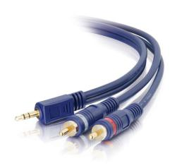
Specifically designed to provide quality music transfer from your PC sound card, portable CD player, MP3 player, iPod®, or any mini-stereo audio device to another audio device with RCA audio jacks. This cable features two 27 AWG oxygen-free copper conductors, a drain wire, an aluminum foil shield to prevent unwanted EMI/RFI interference, and fully molded, gold-plated connectors providing strain relief for a quality connection.
