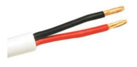
This is the right cable to install audio throughout your house. Made from 41 strands of 99.9% high-purity copper, this speaker wire is very flexible and less likely to kink during installation. CL2-rated for use inside walls, this wire features a flame-retardant white PVC jacket that helps to diminish the potential of fire spreading between floors.
