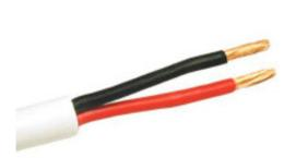
This is the right cable to install audio throughout your house. Made from 41 strands of 99.9% high-purity copper, this speaker wire is very flexible and less likely to kink during installation. CL2-rated for use inside walls, this wire features a flame-retardant white PVC jacket that helps to diminish the potential of fire spreading between floors.
