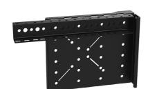
Vertical wall mount fixed 4RU adjustable mounting rail kit. 4RU mounts into both 4RU and 8RU frames. The mounting rails can mount equipment using 10-32 hardware, or can be reversed to also mount with any thread size cage nuts.
